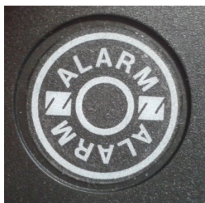
Alarm LED on the controller lid.
